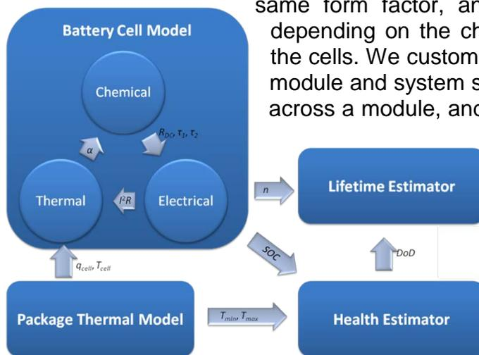
Figure 1: Diagram of a Pack Model
